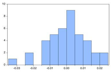
The above graph shows a normal distribution of error terms. Further, we can also check the statistics provided in the above diagram. The probability value of Jarque-Bera is 0.466. So, the null hypothesis was not rejected and it was assumed that errors are normally distributed.
